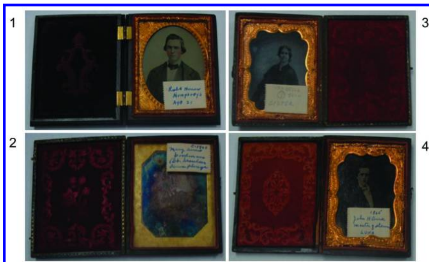
Figure 6. Four daguerreotypes within their cases that were examined for the H 2 S concentrations in the interior microenvironment with Ag NP films.
