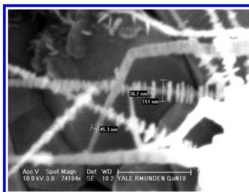
Figure 16. GaN nanowires grown on alumina show dramatic modulation of diameter along the length of the nanowire, perhaps due to fluctuations in source arrival or temperature variations. Diameter varies from ~150 nm to only ~35 nm.
