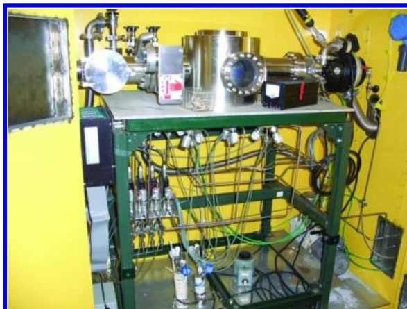
Figure 7. Custom designed chemical beam epitaxy (CBE) system for semiconductor nanowire growth at Yale University.
